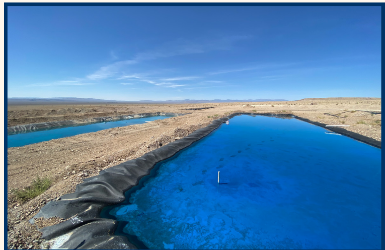
Heap leach pad evaporation ponds at Pathfinder Tonopah's Liberty Mine, which will enhance fluid-inventory solution management, Nye Co., Aug. 2023.
